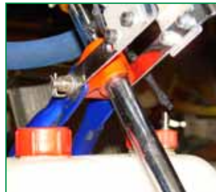
Put a mark on the steering shaft and upper steering support to identify straight ahead. This will be important when scaling your kart.
