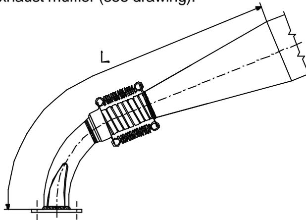
To achieve this dimension, the flexible (supplied with the engine) must be cut at a length of 65mm (flexible completely closed).
