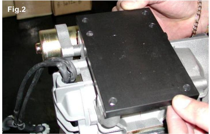
**3.3.3** INSTALL THE MOTOR MOUNT. MAKE SURE TO USE M8 ALLEN SCREWS WITH A LENGTH SUCH AS TO ENGAGE, IN THE CRANKCASE, A THREADED PORTION LENGTH OF 16÷19mm (THE SCREW MUST PROTRUDE FROM THE PLATE FOR 16÷19mm) (SEE FIG. 3 AND DRAW. PAG. 9)
