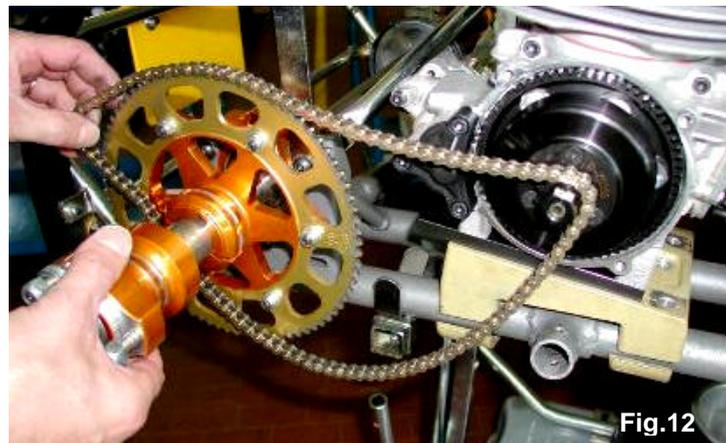
3.5.4 MOVE THE ENGINE ON THE RAILS AND OPTIMIZE THE CHAIN TENSION .
