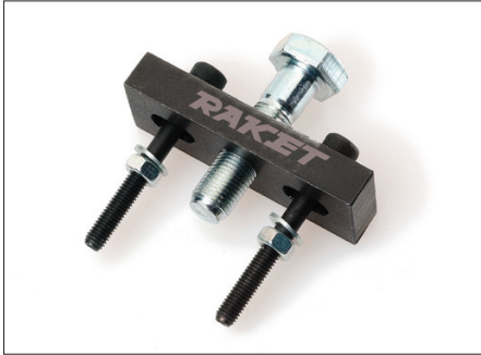
Flywheel extractor for Raket 60, 85 & 120 5051.....
